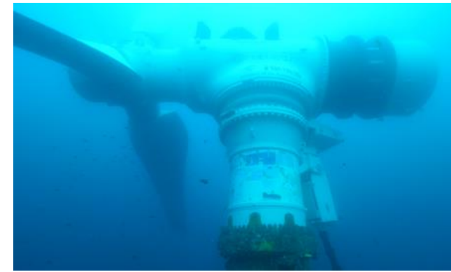
Tidal power generation demonstration project with Ministry of the Environment (Nagasaki Prf., 1,100kW)
